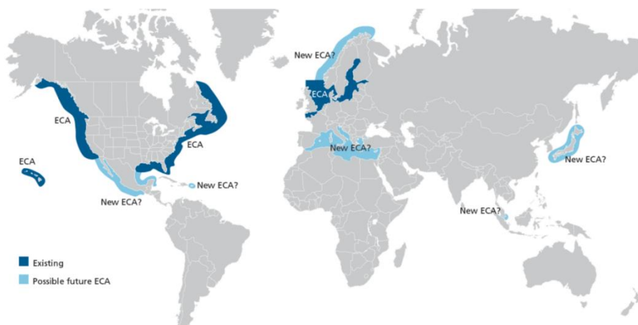
Figure 2-2: Existing and future ECAs for sulphur limit regulations [4]. Used with permission from DNV-GL
