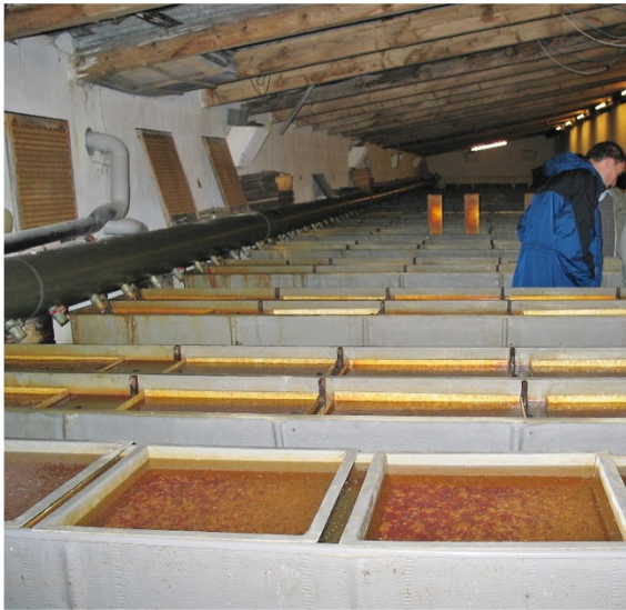
Figure 19: Rainbow trout hatchery facilities: egg incubation, larval rearing units and fingerling growing units using flow-through systems
