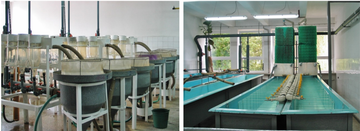
Figure 24: Common carp hatchery: egg incubation and hatching unit, larval rearing unit
